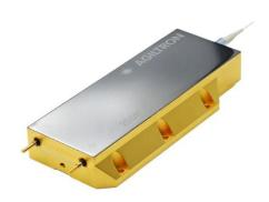
The FCMH series diode lasers deliver up to 500 W of power through a 200 µm fiber. They provide high brightness and simplified thermal management by distributing the diodes (heat sources), allowing for a water-cooled architecture with reliable, predictable performance. A turn-key benchtop unit is available, integrating the power supply, water cooling, power control, and safety shut-off features.
